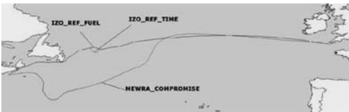
Figure 14. Output of the algorithm MEWRA_COMPROMISE compared to the time-optimal and fuel-optimal isochrone routes for Halifax – Plymouth voyage, departure 2008-02-15 12:00.
