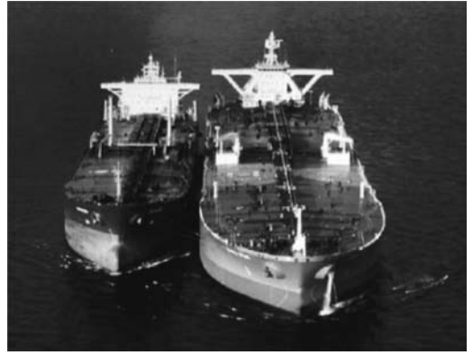
Figure 1. The two ships have come alongside and commenced mooring operation while still underway at slow forward speed. The ships will be brought dead in the water and the STBL is to anchor if the operation takes place in a lightering zone with shallow waters.
