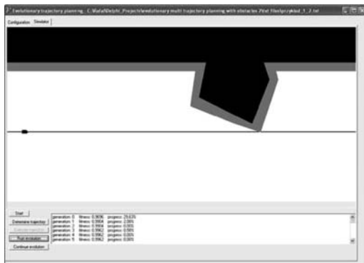
Figure 1. The own ship's current course does not collide with the landmass (black) or its domain (grey).
