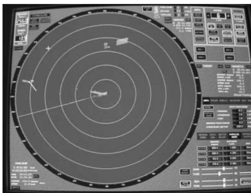
Figure 3. The ARPA simulation displays a 'true' vector from the acquired target on ALMANAMA's starboard bow.
