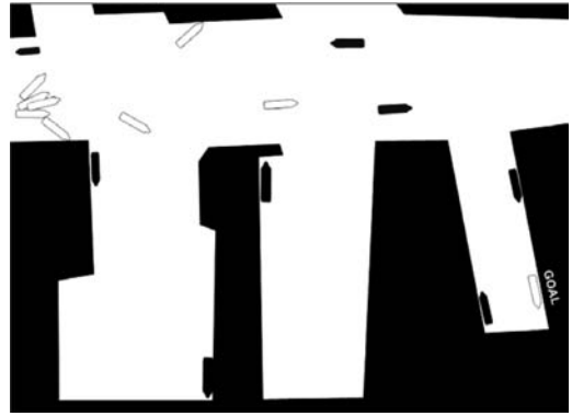
Figure 3. Multi-agent simulation system. Helmsmen compete with each other simultaneously to find the optimum route to goal.
