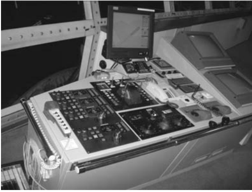
Figure 2. View of m/f “Polonia” manoeuvring controls on port side wing.
