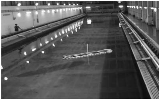
Figure 10. Zig-zag test in towing tank.
