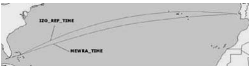
Figure 6. Output of the algorithm MEWRA_TIME compared to the time-optimal isochrone route for Lisbon-Miami voyage, departure 2008-09-02 00:00.
