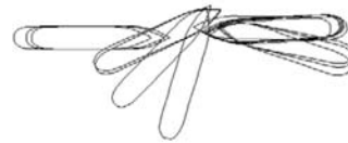
Figure 12. The turning manoeuvre, portside turn, with current 090° and 2 knots – ship shapes in time of commands.
