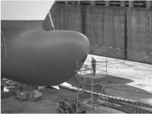
Figure 4. Transducer usually is mounted in the bow.
