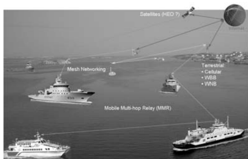
Figure 8. Illustration of the suggested ‘Wireless Coastal Area Network’ (WiCAN) concept.
