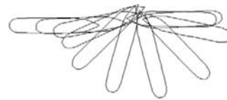
Figure 13. The turning manoeuvre, portside turn, with current 090° and 2 knots – ship shapes in every 30s.
