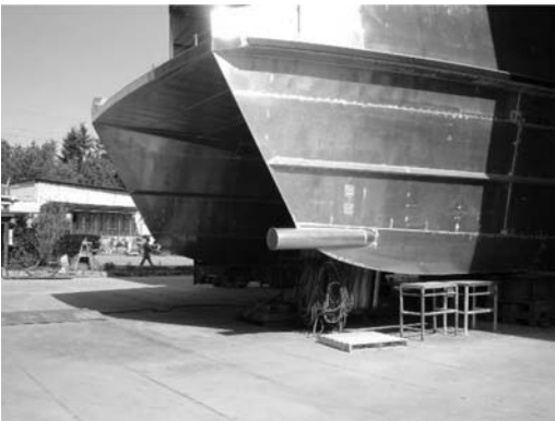
Figure 13. Transducer installed on the bow of a hulk.
